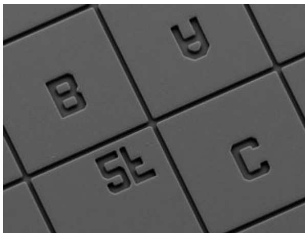
Hot embossing is used to imprint microscale structures in thermoplastics. A biomedical device
