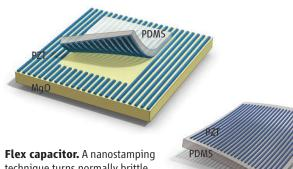
Flex capacitor. A nanostamping technique turns normally brittle PZT into flexible nanowires encapsulated in a rubber sheet.
