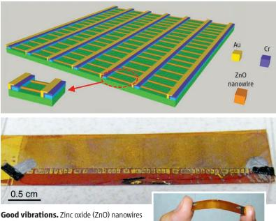
are grown between chromium (Cr) and gold (Au) electrodes (top) to make a nanogenerator that produces a high voltage when flexed.
