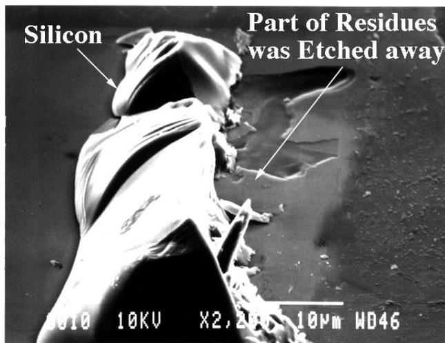
Fig. 6. Enlarge view showing the square box portion of Fig. 5 after the sample was immersed in gold etchant for 30 minutes. Part of the residues were etched away due to the diffusion of gold into the silicon substrate.
