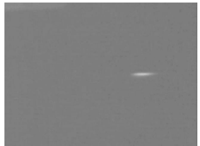
Fig. 7. Hot spots are shown under the Joule heating effects when the light on the optical microscope is turned off.
