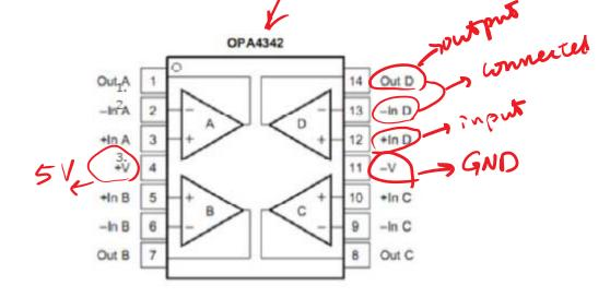
Verify that there is unity gain or Vin = Vout for your voltage follower. You can easily do this by connecting the wiper of your potentiometer, which has been connected between 5V and ground, to the non-inverting input (+ In C), The wiper is the part that changes voltage as the knob turns.
