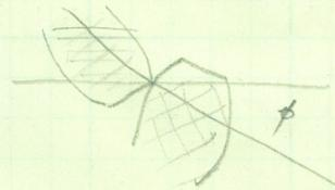
⇒ contact starts when addendum circle of driven gear intersects the pressure line
