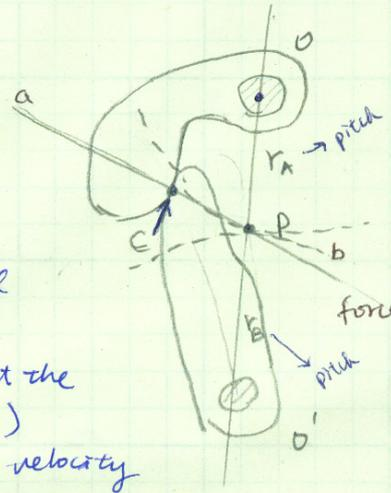
$C$  is the contact point where two surfaces are tangent to each other
