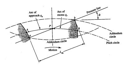
for a short period of time, there will be two teeth in contact, one in the vicinity of A and another near B. As the meshing proceeds, the pair near B must cease contact, leaving only a single pair of contacting teeth, until the procedure repeats itself.
