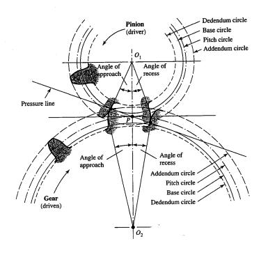
To draw a tooth, we must know the tooth thickness. From Eq. (13-4), the circular pitch is
