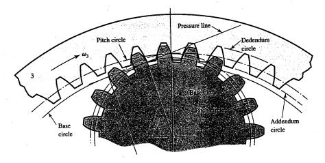
Thus the pitch circles of gears really do not come into existence until a pair of gears are brought into mesh.
