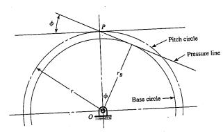
Next, on each gear draw a circle tangent to the pressure line. These circles are the base circles. Since they are tangent to the pressure line, the pressure angle determines their size. As shown in Fig. 13-10, the radius of the base circle is
