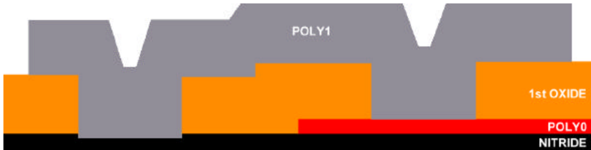
Figure 2.19. Poly 1 properly overlaps ANCHOR1 holes to prevent attack of underlying films as seen in figure 2.18. By completely overlapping the anchor holes, the maximum topography is also reduced (see fig. 1.1 for fill patterns).
