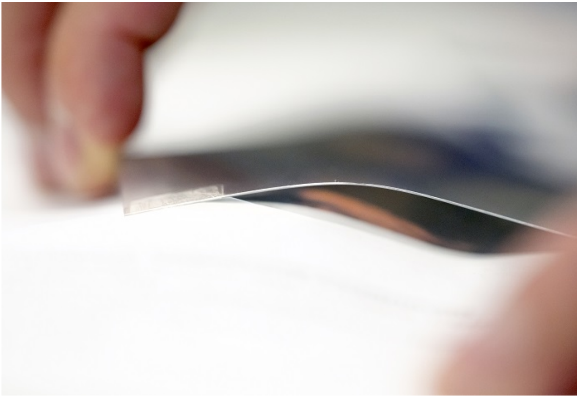
The sensor-actuator patch is about 150 \mu\text{m} thick, similar to the diameter of a human hair. (Image: Adam Lau, UC Berkeley College of Engineering)
