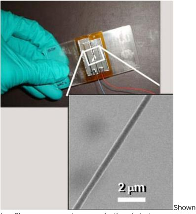
is a fiber nanogenerator on a plastic substrate created by UC Berkeley scientists. The nanofibers can convert energy from mechanical stresses and into electricity, and could one day be used to create clothing that can power small electronics. (Chieh Chang, UC Berkeley)
