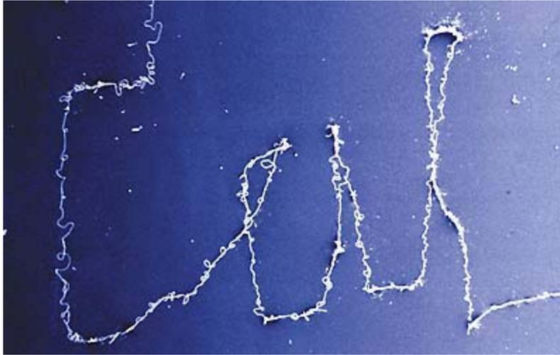
Grad student Chieh Chang wrote the word "Cal" using a new electrospinning technique developed in Liwei Lin's laboratory at UC Berkeley. Ron Wilson photos
