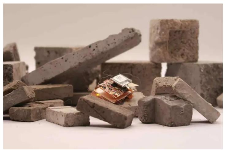
The robot is built of a layered material that bends and contracts when an electric voltage is applied, allowing it to scurry across the floor with nearly the speed of an actual cockroach. (UC Berkeley photo courtesy of Jiaming Liang & Liwei Lin)
