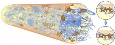
Fluorescent tetrapod quantum dots or tQDs (brown) serve as stress probes that allow precise measurement of polymer fiber tensile strength with minimal impact on mechanical properties. Inserts show relaxed tQDs (upper) and stressed tQDs (lower).
