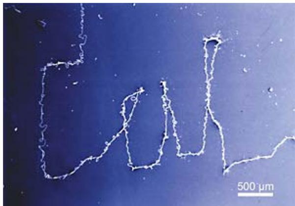
**Liwei Lin and colleagues used near-field electrospinning to spell “Cal,” demonstrating that nanofibers could be deposited in a controlled manner rather than the tangled mass resulting from earlier methods. The technique has potential for producing specialized wound dressings and chemical detectors.**
