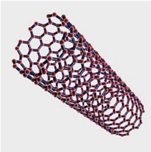
Carbon nanotubes measure only a few nanometers in diameter. With their extraordinary strength, efficient thermal conductivity and high surface-area-to-volume ratio, they have multiple potential applications in electronics, optics and materials science.
