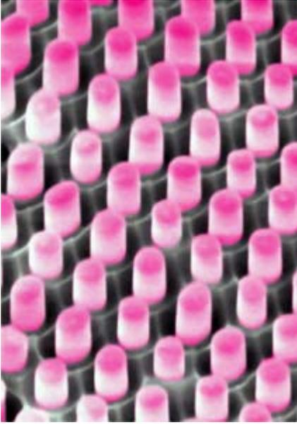
This scanning electron microscopic image of single-crystalline nanopillar cells of optically active semiconductor on aluminum substrate, grown by Ali Javey (EECS) and his team, could facilitate production of highly efficient and cost-effective photovoltaic solar cells.
