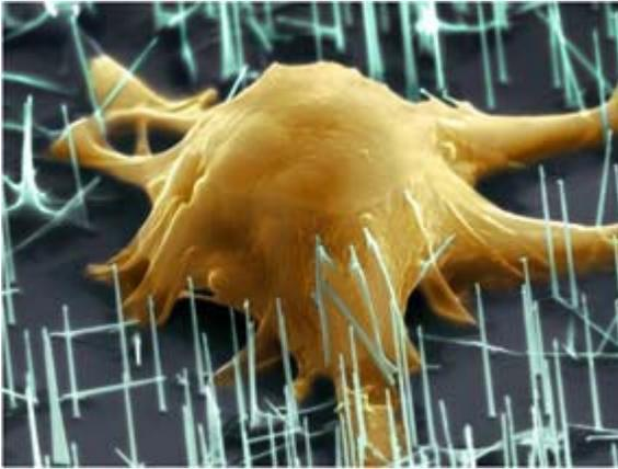
**This scanning electron microscopic image shows a mouse embryonic stem cell cultured on an array of silicon nanowires, the work of Peidong Yang (Chemistry, MSE). The wires measure from 1 to several hundred nanometers across, the cell about 10 micrometers.**
