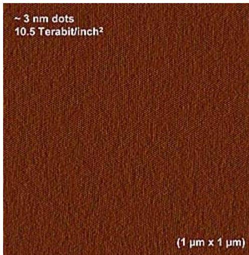
**This atomic force microscope image shows a highly ordered arrangement of nanoscale dots, each just 3 nanometers in size. The ultra-dense material, the work of Ting Xu (MSE) and colleagues, could make it possible to store the contents of 250 DVDs in an area the size of a U.S. quarter.**
