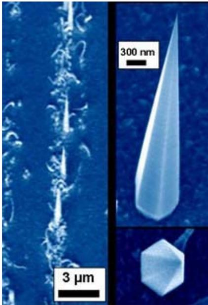
This gallium arsenide nanoneedle is the sharpest point she's seen, says Connie Chang-Hasnain (EECS), who discovered it on silicon while exploring methods to monolithically integrate dissimilar single crystals. The nanoneedle has the capacity to convert single photons into more than 100 cascades of electrical charge, giving them potential as both optical detectors and solar cells.
