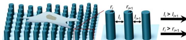
**Figure 1** Microfabricated post array with decreasing interpost spacing ( $I$ ) and decreasing radii ( $r$ ) from post-to-post
